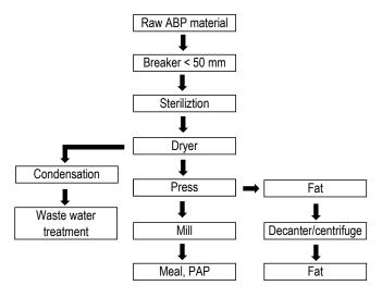
Figure 1. General scheme of rendering production flow chart for animal by-product (ABP) material (Alm, 2012a). PAP – processed animal protein
