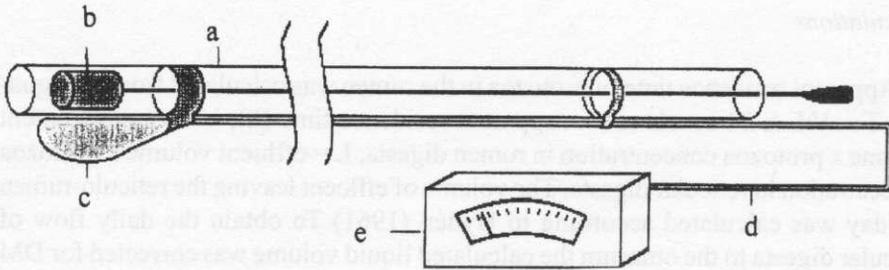
Figure 1. Device construction for collection of the reticular digesta *via* rumen cannula. a – collecting tube; b – rubber piston; c – ballon; d – connecting tube; e – recording apparatus
